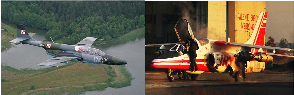
Figure 3: The jet trainers: TS-11 Iskra (Spark) on the left and PZL I-22 on the right
